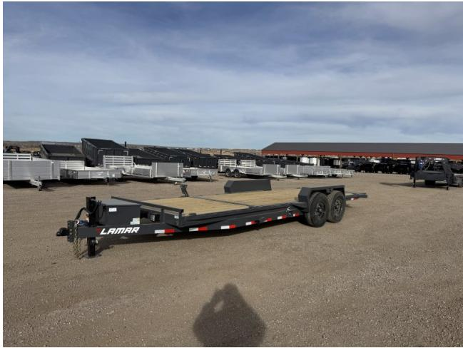
**\$10,995****Stock #:** LM4701**VIN/Serial:** 5RVBT2228TP150921**Category:** Equipment**Cond.:** New**Year:** 2026**Make:** Lamar**Model:** 83X22 15.6K TILT 14 PLYS**Color:** Gray**Width:** 83" **Length:** 22'**GVWR:** 15,680
